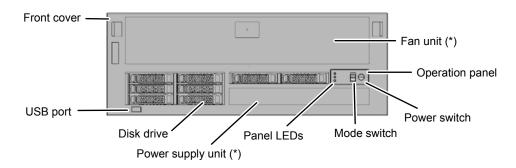
\*: You can see the fan unit and the power supply unit by removing the front cover.
